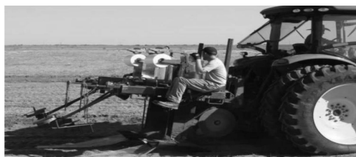
Figure 1. SWRT membrane installation equipment (Smucker and Basso, 2014).
