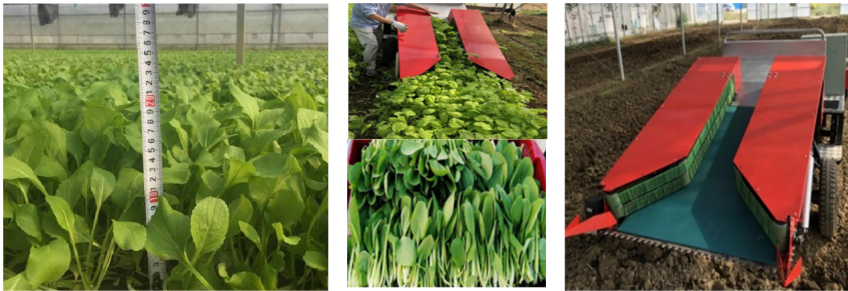
(a) Appearance of small green vegetables to be harvested (b) Harvesting process and effects (c) Structure diagram of intelligent harvester prototype
