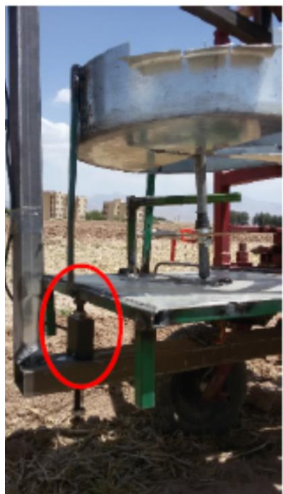
Figure 5. Load cell installation on prototype under YMS.
