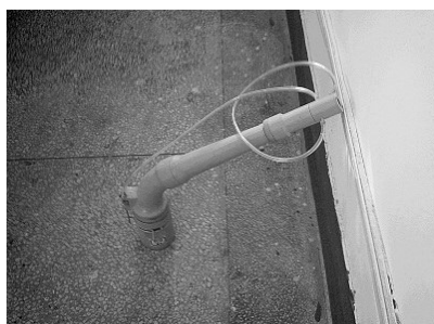
(a) The new type of fluidic sprinkler
