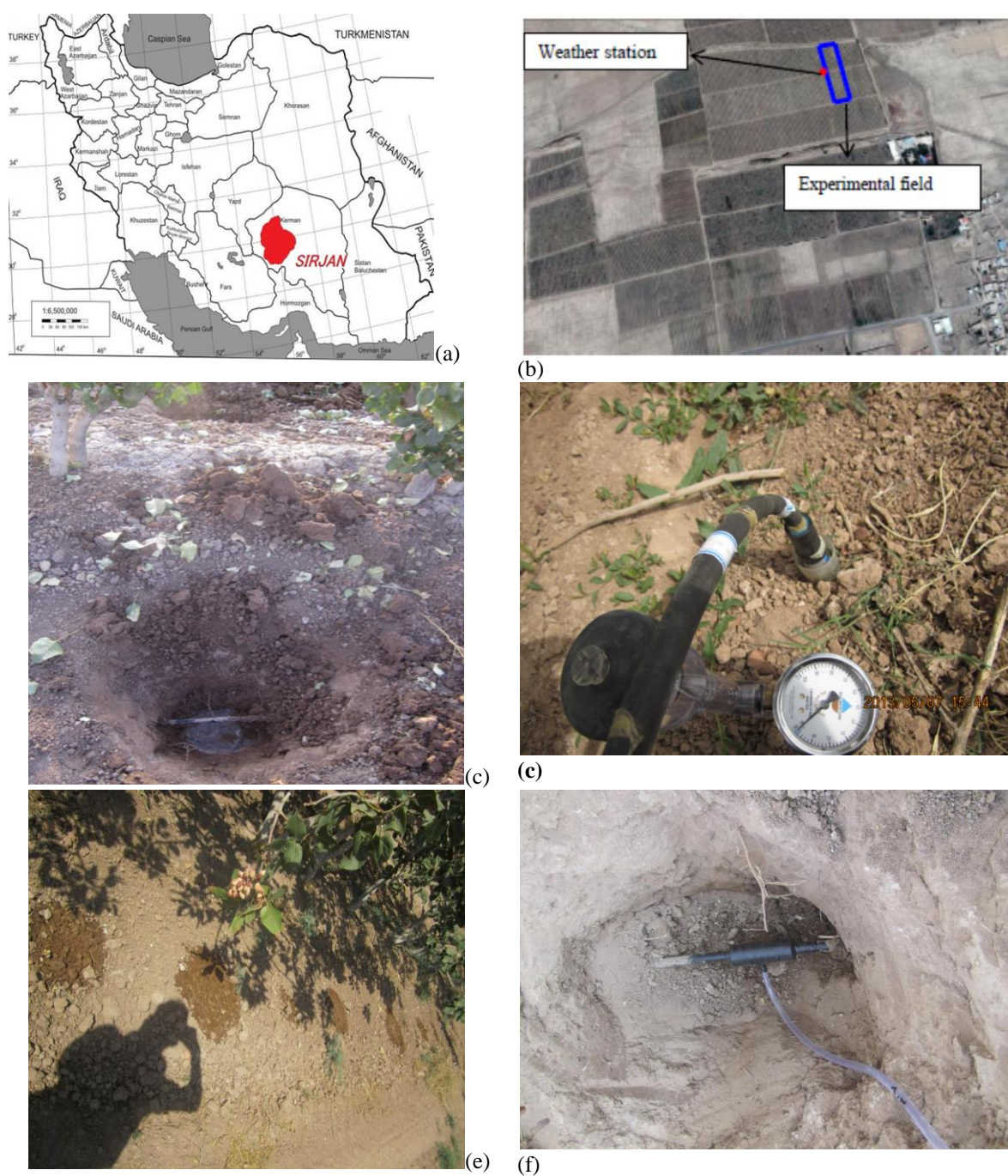
Figure 1. (a) Experimental site in Kerman Province (Sirjan City), (b) Experimental trees rows and the private weather station at 90 ha pistachio orchard, (c) Water flow from subsurface emitters, (d) Soil moisture measurement using TDR, (e) Surface wetting pattern from subsurface emitters, and (f) Air injection measurement .
