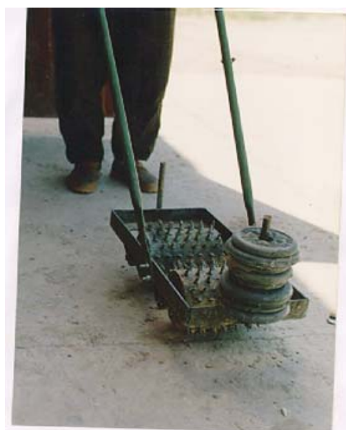
Figure 4. Crust breakers: (a) rolling cultivator and (b) manually operated rolling-type soil crust breaker.
