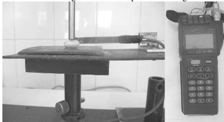
Figure 4. Instruments employed to measure Poisson's ratio for unsplit pistachio nuts.
