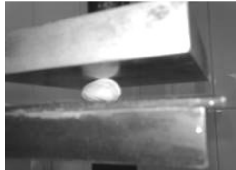
Figure 1. Direction of loading in quasi-static compression test of unsplit pistachio nut using parallel plates.
