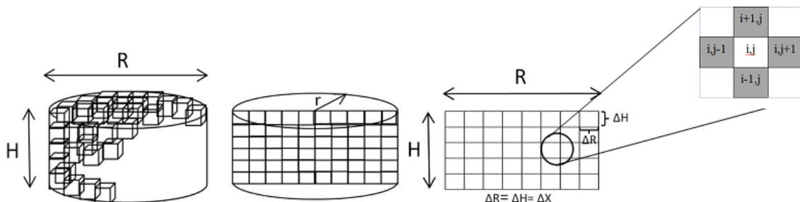
**Figure 1.** Inverting 3D cylinder to a 2D in case of axial symmetrical problem and Von Neumann neighborhood (Kier *et al.*, 2004; Luikov, 1968).
