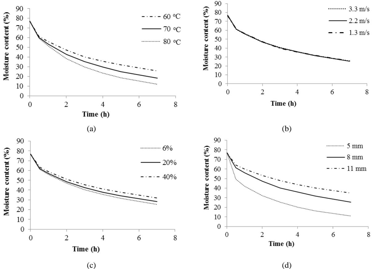
**Figure 3.** Model results of cellular automata for the effect of (a) drying air temperature (b) air flow velocity (c) relative humidity (d) sample thickness, on moisture content during hot air drying ( $V=3.3 \text{ m s}^{-1}$ ,  $RH=6\%$ ,  $Th=8 \text{ mm}$ ).
