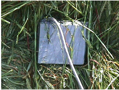
Figure 12. extended octagonal ring sensor placed inside the bale.
