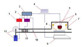
**Figure 1**. Schematics of the experimental dryer coupled with the image recording system: (1) Inverter; (2) SSR rely; (3) D/A transducer; (4) Computer; (5) Camera; (6) Florescent lamp; (7) Fiber glass; (8) Thin layer grapes; (9) Balance; (10) Temperature sensor; (11) Heater, (12) Fan and electromotor.
