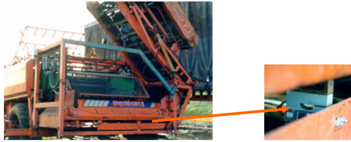
Figure 12. Diagram of the load cell supporting system in the potato harvester.
